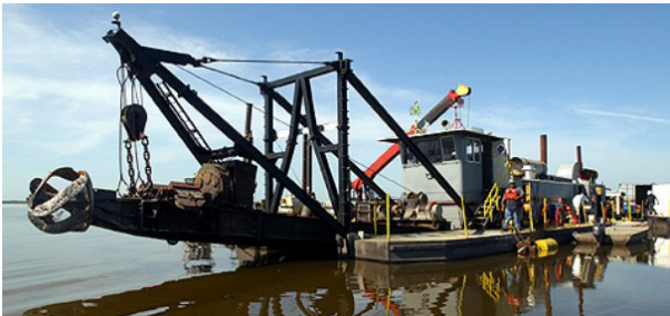
Fig. 2.22 A typical hydraulic dredging operation. Photo: www.naplesnews.com .
