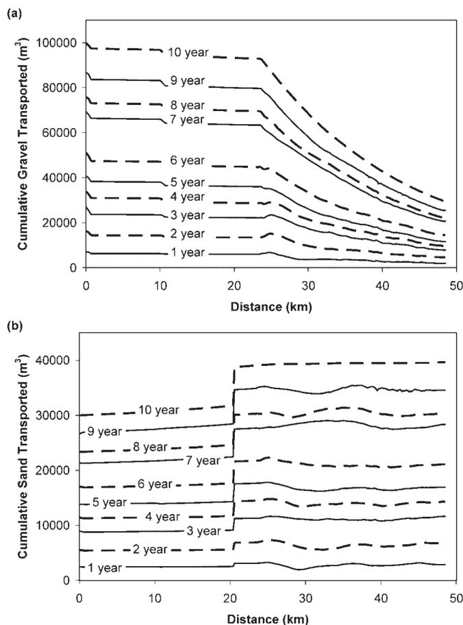
Figure 8. Simulated (a) cumulative gravel transport and (b) cumulative sand transport, Run 1. The decreasing volume of gravel transport in the downstream direction is due to the abrasion of gravel and the lack of tributary input, and the increasing volume of sand transport in the downstream direction is due to gravel abrasion, which produces a small fraction of sand and a large fraction of silt and clay, and the contribution from the Bull Run River at 20.5 km
