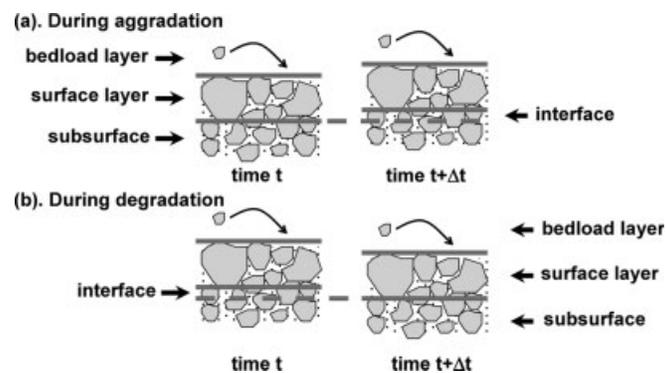
Figure 2. The three-layer conceptual model, adapted from Parker (1991a,b), used in TUGS model, showing the bedload, surface and subsurface layers. A fourth layer, the interface layer, exists only conceptually because its thickness  $\rightarrow 0$  when time interval  $\Delta t \rightarrow 0$ . A hypothetical sand transfer function was used in TUGS model, linking interface layer sand fraction to surface layer sand fraction for sand exchange during channel aggradation
