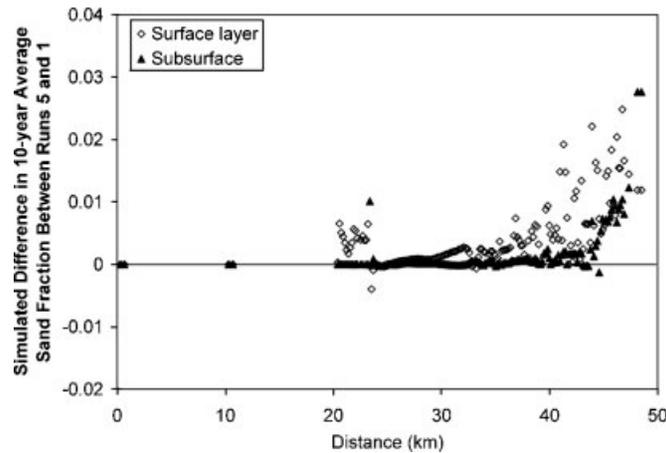
Figure 15. Simulated surface and subsurface sand fraction for Run 5, presented as changes from that of Run 1
