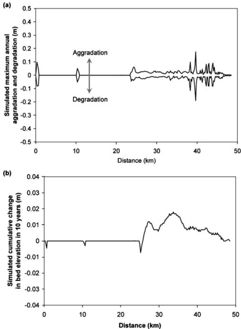
Figure 7. Simulated 10-year period channel bed variation for Run 1: (a) maximum annual aggradation and degradation; and (b) cumulative change in bed elevation in a 10-year period
