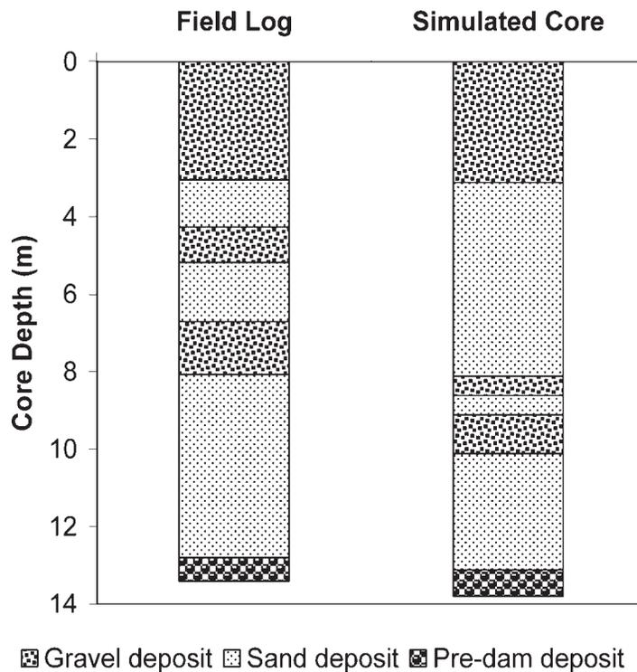
Figure 17. Comparison of simulated sediment texture in the core indicated in Figure 16(b) with field log from a core located at proximity of the simulated core. The differences in the vertical location of the gravel lenses are most likely due to the fact that there was no event-by-event sediment supply information available for the modelling exercise
