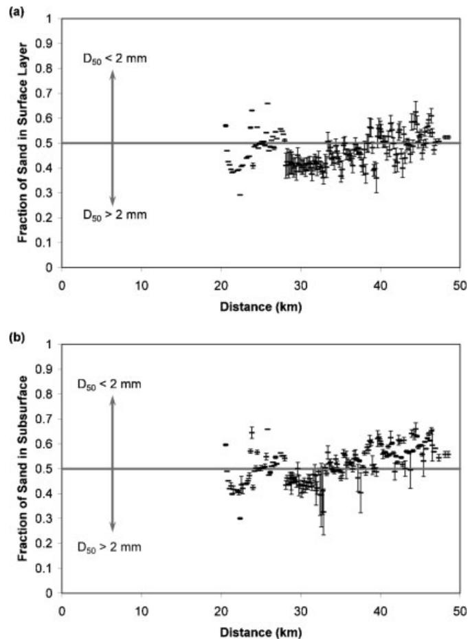
Figure 12. Simulated (a) surface and (b) subsurface sand fraction for Run 6
