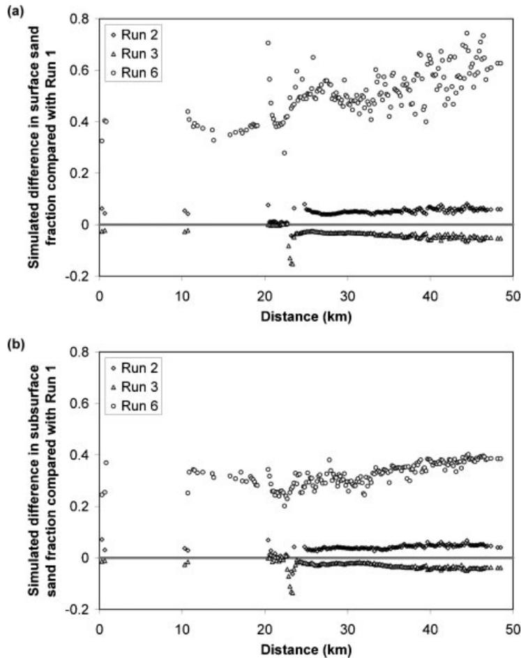
Figure 11. Simulated (a) surface sand fraction; and (b) subsurface sand fraction for Runs 2, 3 and 6, presented as differences from that of Run 1
