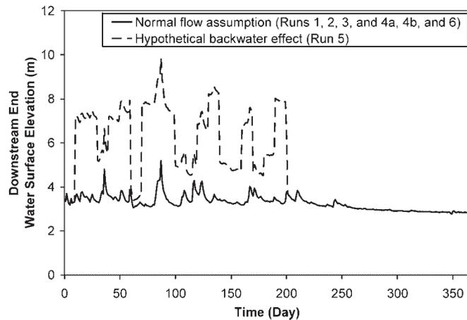
Figure 14. Assumed backwater effect at the Sandy River–Columbia River confluence (i.e. downstream end of the study reach) for Run 5
