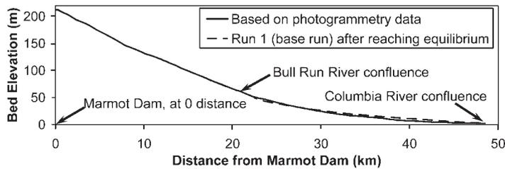
Figure 4. Longitudinal profile of the Sandy River downstream of Marmot Dam, compared with TUGS model simulation, Run 1
