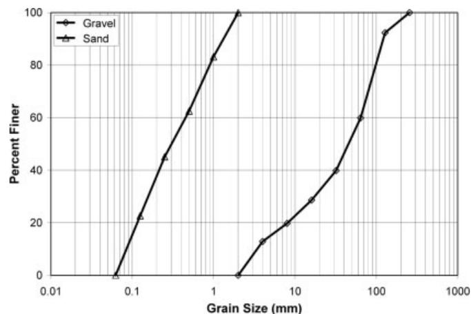
Figure 5. Estimated gravel and sand grain size distributions in sediment supply, based on coring data of Marmot Reservoir sediment deposit
