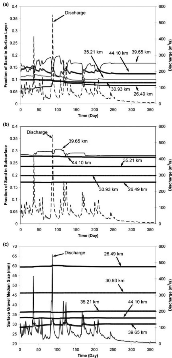
Figure 10. Predicted evolution of grain size characteristics at five locations: (a) surface sand fraction; (b) subsurface sand fraction; and (c) surface median size (excluding sand)
