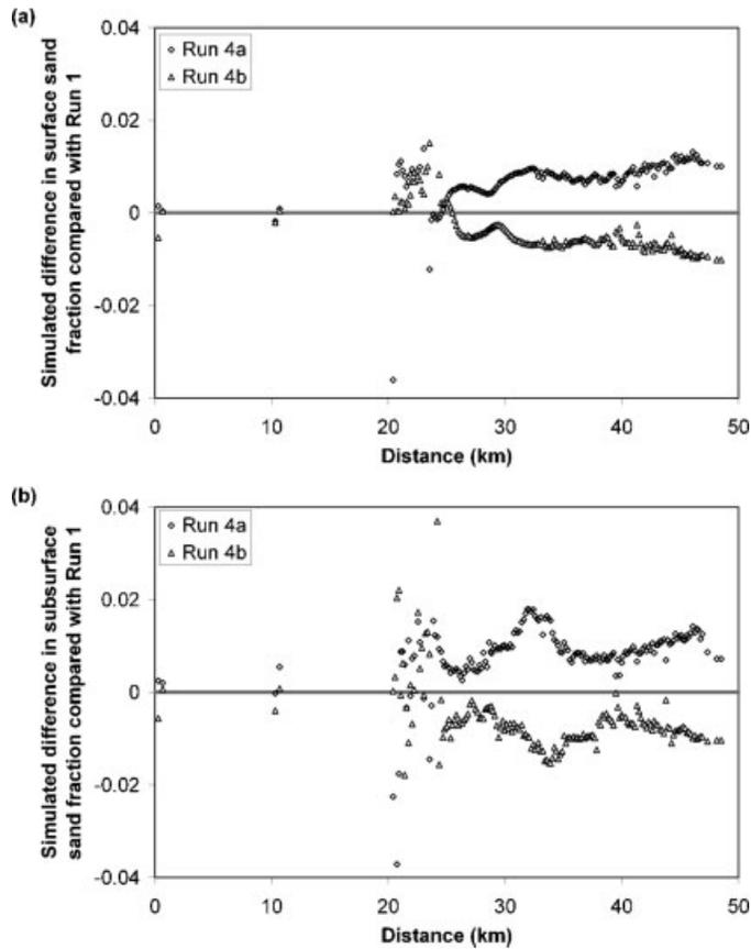
Figure 13. Simulated (a) surface sand fraction; and (b) subsurface sand fraction for Runs 4a and 4b, presented as differences from that of Run 1
