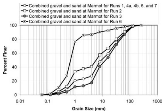
Figure 6. Assumed grain size distributions for combined gravel and sand in sediment supply for all the runs
