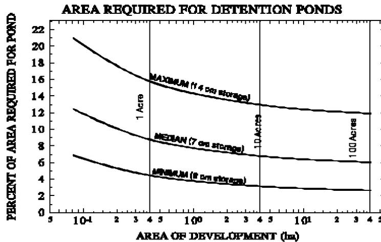
**Figure 7.** Relative gross area required for detention ponds, depending on the development area and the desired volume of stored runoff (expressed as cm-ha per ha of developed land). Pond layout and design is in accord with local regulations and assumes a 1.3-m (4-ft) maximum water depth and 3:1 sideslopes on all confining berms. Range of pond volumes correspond to the likely values determined with a “KCRTS duration” standard (Figure 6).
