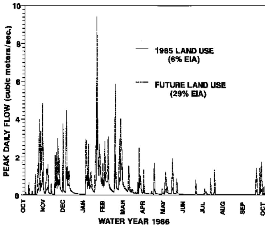
**Figure 2.** One year of simulated streamflow from a 14.2-km<sup>2</sup> watershed (Soosette Creek), under identical rainfall but differing land uses, using the continuous numerical model HSPF (USEPA, 1984). Parameters characterize the present-day (1985) land cover (6 percent effective impervious area
